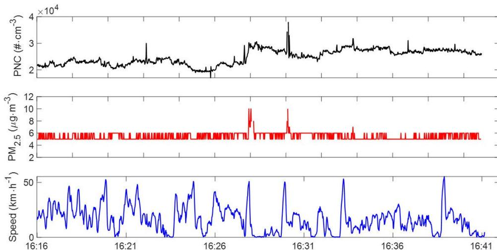
**Fig. 2.** Time series of PNC (particle number concentrations), PM<sub>2.5</sub> concentrations, and mobile platform speed measured on the rarely trafficked road (inside the Pukyong National University campus). The spikes in PNC and PM<sub>2.5</sub> time series were from intermittently-encountered vehicles/motorcycles.
